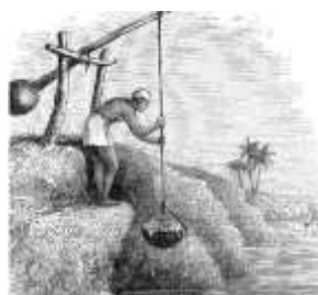
Figure 2 An AI-generated image of water raised using a Shaduf, as suggested by Verner (2014)
