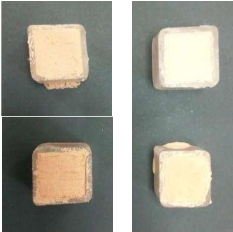
Fig (13) microballoon 1, microballoon 2, microcrystalline2 and microcrystalline3 after drying in acrylic molds
