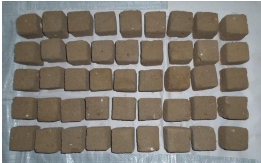
Fig.1 mudbrick samples (5x5x5) cm prepared accordance to one of the pyramids builders tombs.
