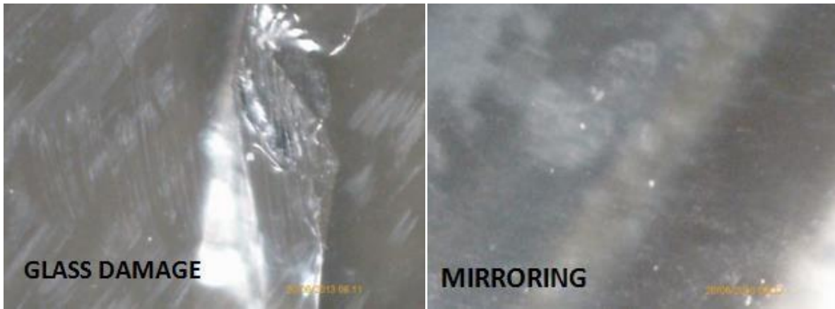
Figure 14. Glass damage (left) and silver mirroring (right).
