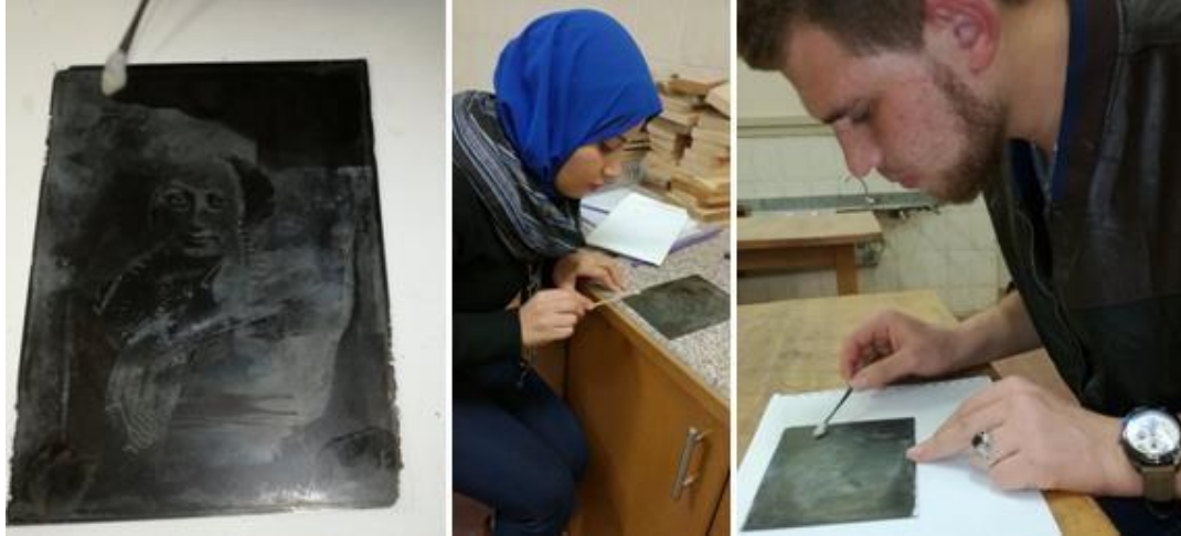
Figure 17. Silver mirroring reduction using solvent cleaning.
