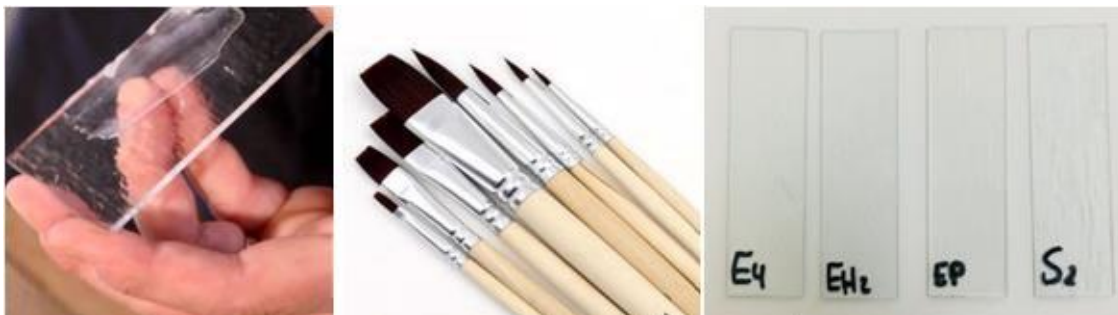
Figure 3. Applying adhesives to glass slides by brush.
